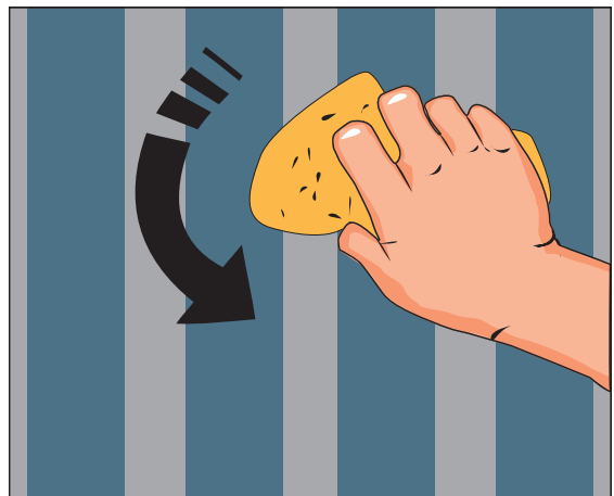
Any paste spilled on the front of the wallpaper must be carefully removed immediately using a soft, damp wallpaper sponge.
