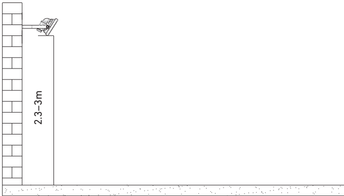
Fig 2. Mounting instructions for LED spotlight (without movement detector)
