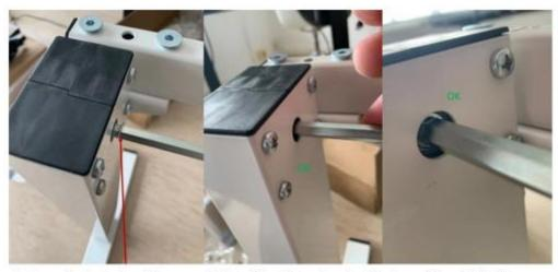
The transmission shaft must be secured to the fixed washer at the bottom of the post/leg. (It is not properly attached in this picture.)
